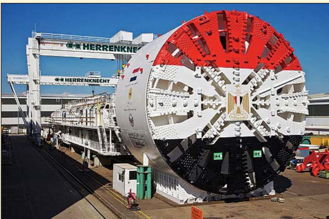
Obr. 5 Mixshield Herrenknecht Ø 13,02m
