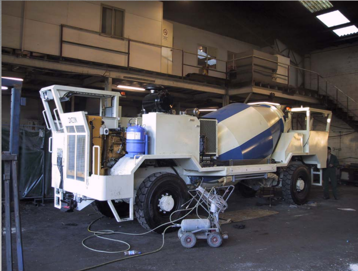
Concrete Truck – 5m 3 capacity
