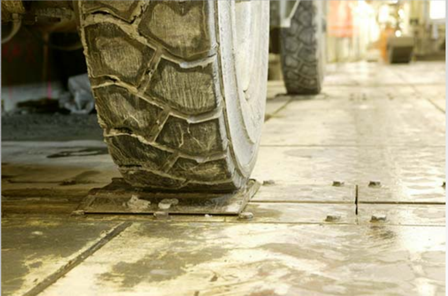
Rubber Tired Agitator Truck – Detail of Sliding Deck
