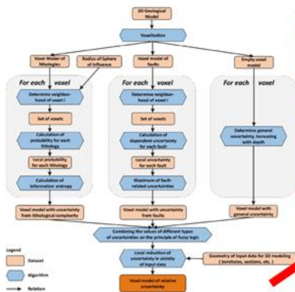
Fig. 4 Diagram of the workflow of the determination of the uncertainty of 3D geological models, including the related algorithms. Legend: orange - input data, blue - algorithm, brown - final output
