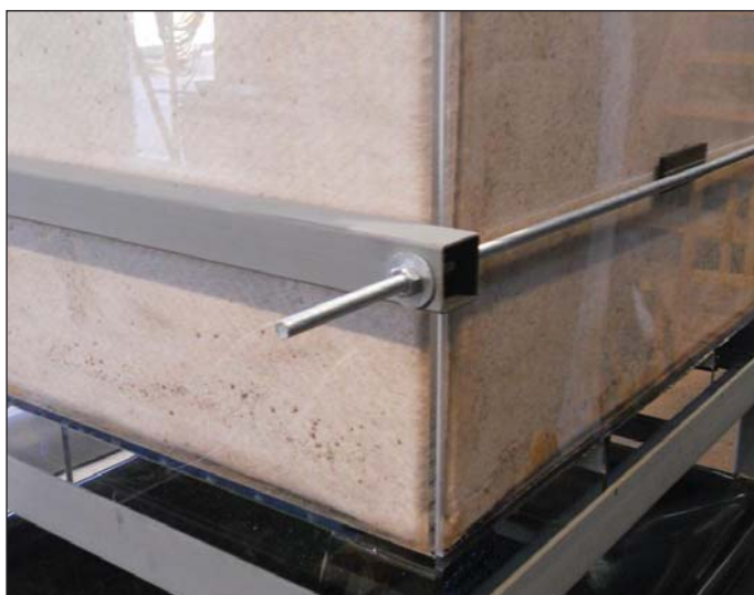
Obr. 10 Zkouška funkce izolace VOLTEX (typ 2) – detail po napuštění nádoby vodou Fig. 10 Testing of VOLTEX waterproofing material function (type 2) – a detail after the filling of the vessel with water
