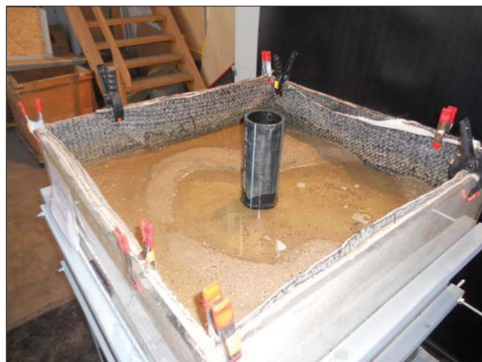
Obr. 9 Zkouška funkce izolace VOLTEX (typ 2) – nádoba po napuštění vodou Fig. 9 Testing of VOLTEX waterproofing material function (type 2) – the vessel after filling with water
