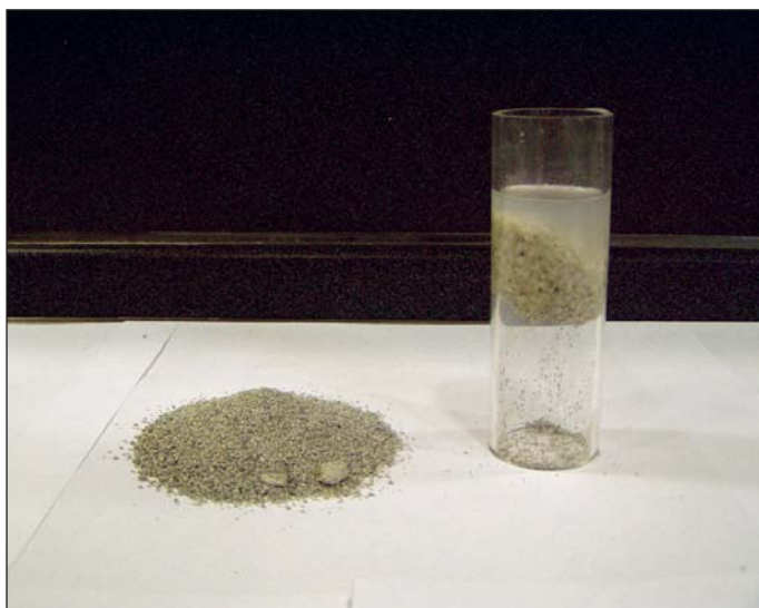
Obr. 1 Princip bentonitové izolace Fig. 1 Bentonite waterproofing principle
