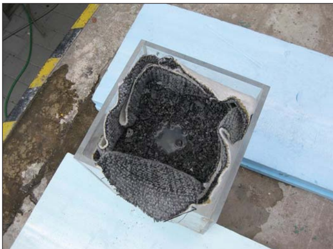
Obr. 5 Zkouška funkce izolace VOLTEX (typ 1) – nádoba po napuštění vodou Fig. 5 Testing of VOLTEX waterproofing material function (type 1) – the vessel after filling with water
