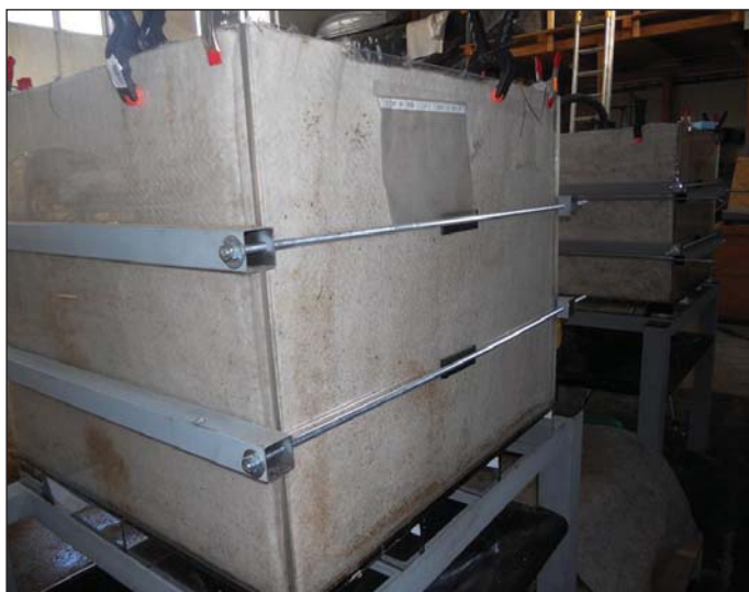
Obr. 7 Zkouška funkce izolace VOLTEX (typ 2) Fig. 7 Testing of VOLTEX waterproofing material function (type 2)
