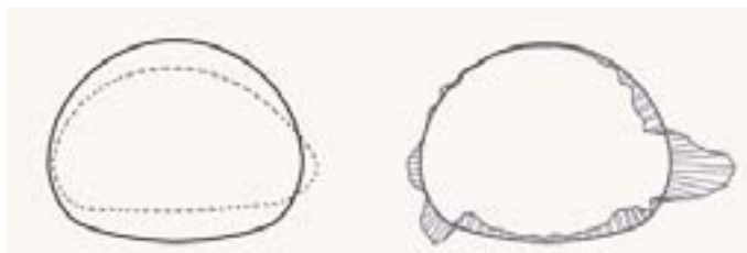
Fig. 5 Deformations of the tunnel lining and distribution of bending moments resulting from a cavern beside the tunnel
