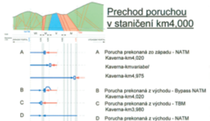
Obr. 3 Možnosti prechodu geologickou poruchou v km 4,000 (3000 m od VP) Fig. 3 Possibilities of passing the geological disturbance at km 4,000 (3000 m from the EP)
