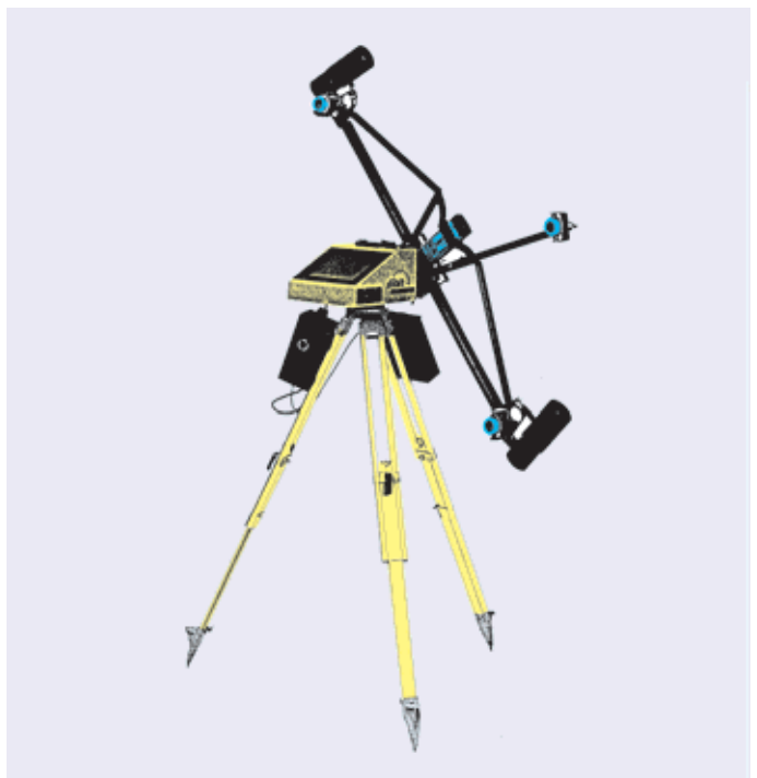
Obr. 2 Tunnelscanner DIBIT Fig. 2 DIBIT Tunnelscanner
