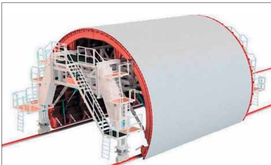
Obr. 8 3D model debniaceho voza Fig. 8 3D model of the formwork truck
