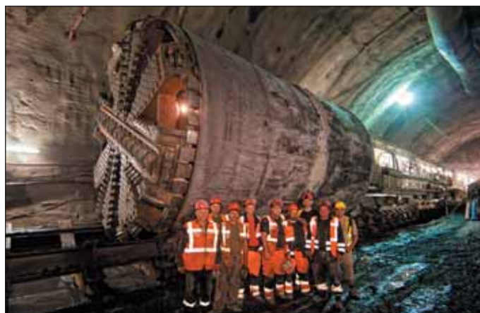
Obr. 11 Štít S-610 ve stanici Bořislavka (2012) Fig. 11 Shield S-610 in the Bořislavka station (2012)
