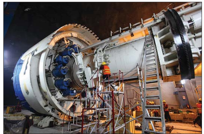
Obr. 3 Plnoprofilové TBM na projektu Neelum-Jhelum Fig. 3 Full-face open type TBM, Neelum-Jhelum Project
