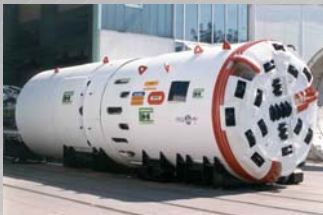
Double Shield-TBM: S-153 La Réunion, \varnothing 3.80m
