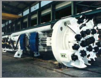
Double Gripper-TBM: S-96 TBM 3000, \varnothing 3.00 m
