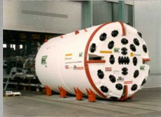
Shielded-TBM with articulation joint: S-163 Sörenberg, \varnothing 4.56 m
